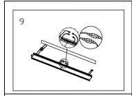
For sharing power between track sections, make wiring connection. If separate power, do not.
