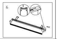
Slide "Track Connector" between sections to interconnect channels.
