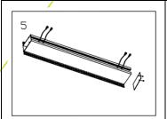
Remove End Cap of second channel if connecting multiple lengths of channel together.
