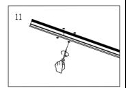
Secure channel system to structural support as necessary assuming worst-case weight of 10 pounds per linear foot.
