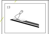
Mud and sand joint compound as needed to create a smooth trimless channel to the ceiling structure.
