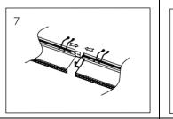
Tighten down Screws to fasten the sections together.
